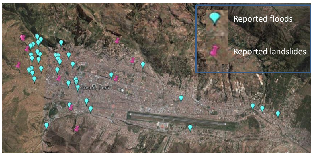
Figure 2.1 Approximate location of floods and landslides reported in the city of Cusco based on the analysis of DesInventar Database (1970s-2011) and placed over a Google earth image. The date of the image is 2008. Most of the data reported in DesInventar have been collected from reports in the media.
